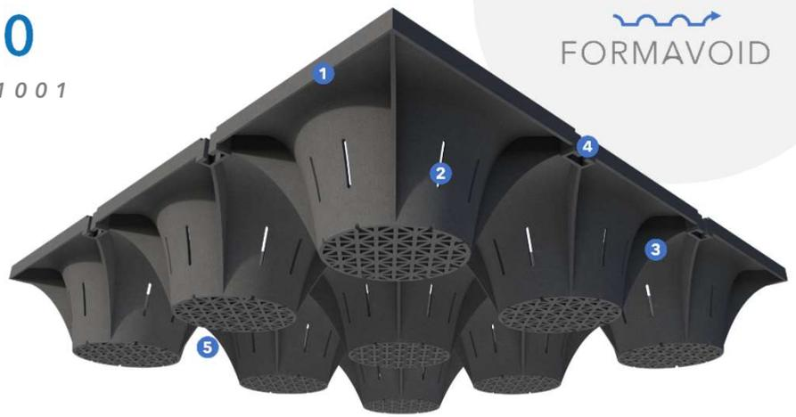
Formavoid is a plastic void former that encourages fill material into an extremely strong series of columns and arches, leaving open void space beneath the arches for source control water management & storage. When filled with aggregates such as MOT Type 3, Formavoid combines with the aggregate to create a granular base with enhanced stability and water storage capacity. A seamless addition and enhancement to source control subbase attenuation.
