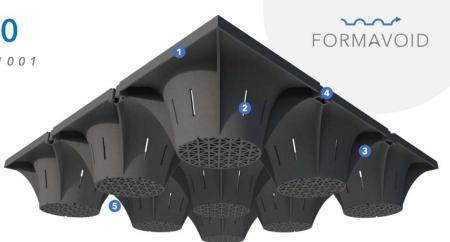
Formavoid is a plastic void former that encourages fill material into an extremely strong series of columns and arches, leaving open void space beneath the arches for source control water management & storage. When filled with aggregates such as MOT Type 3, Formavoid combines with the aggregate to create a granular base with enhanced stability and water storage capacity. A seamless addition and enhancement to source control subbase attenuation.
